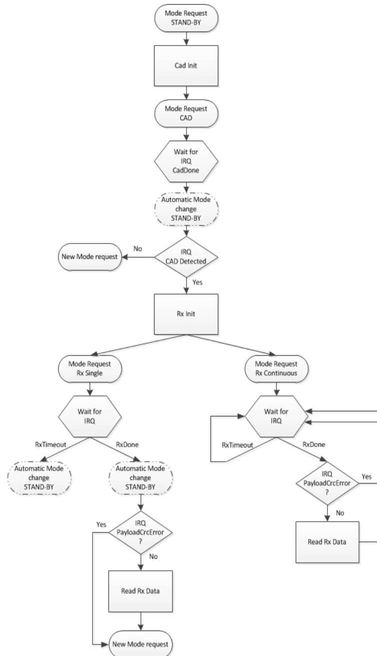
Figure 10. LoRa™ CAD flow
